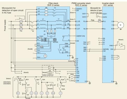
(Note 1) Connect a step-down transport to lower the voltage of the sequence circuit to voltage shown by figure.
