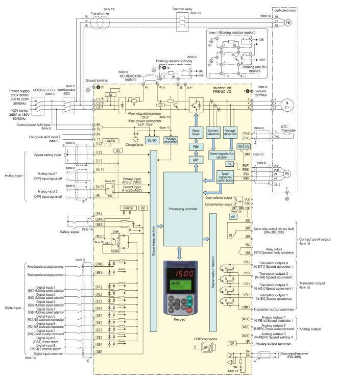
Install a recommended molded-case circuit-breaker (MCCB) or an earth-leakage circuit-breaker (ELCB) with an overcurrent protection function in the primary circuit of the inverter to protect the wiring. At this time, ensure that the circuit breaker capacity is equivalent to or lower than the recommended capacity.
