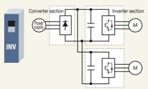
The converter and inverter sections are separately set in this type. The converter (diode stack) or PWM converter is required depending on the intended use. Moreover, a combination of inverters can be used with one converter.
