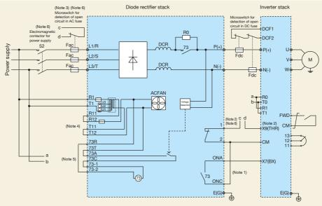
Note 1) Construct a sequence so that the run command is input to the inverter after the initial charging of the diode rectifier has been completed.
